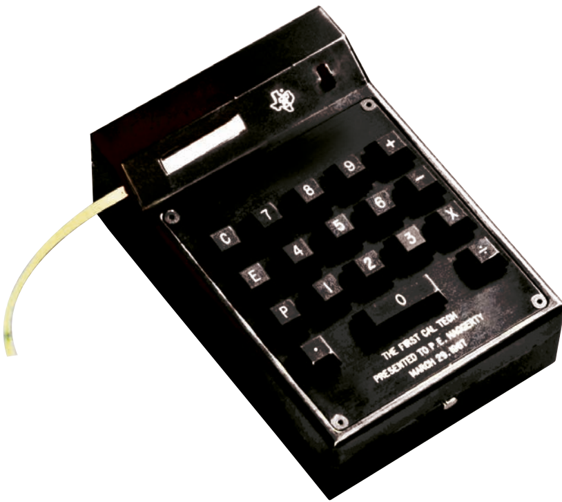
Design model for the CAL TEC calculator from Texas Instruments from 1966/67. The calculator was never marketed.
