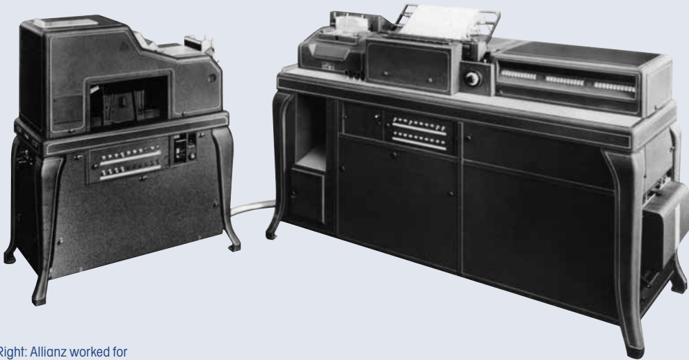
Right: Allianz worked for more than two decades with the D11 tabulating machine, here in combination with the 560 cumulative puncher.
