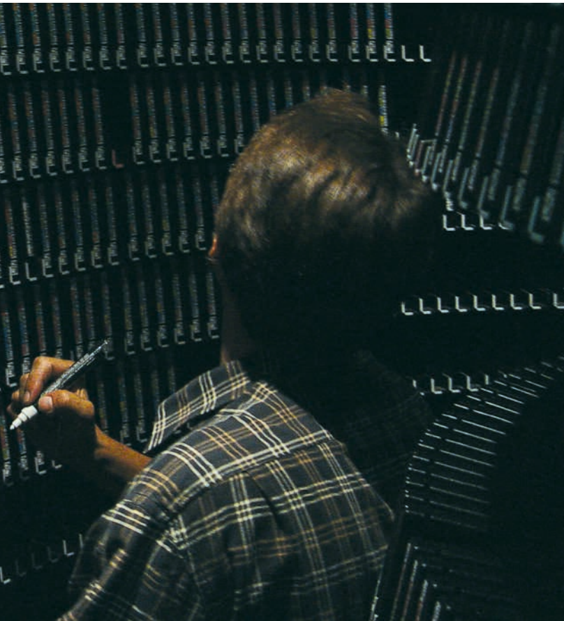
Interior view of a so-called robot silo. An AGIS employee labels cassettes that, among other data storage devices, are used to back up workplace and business data.
