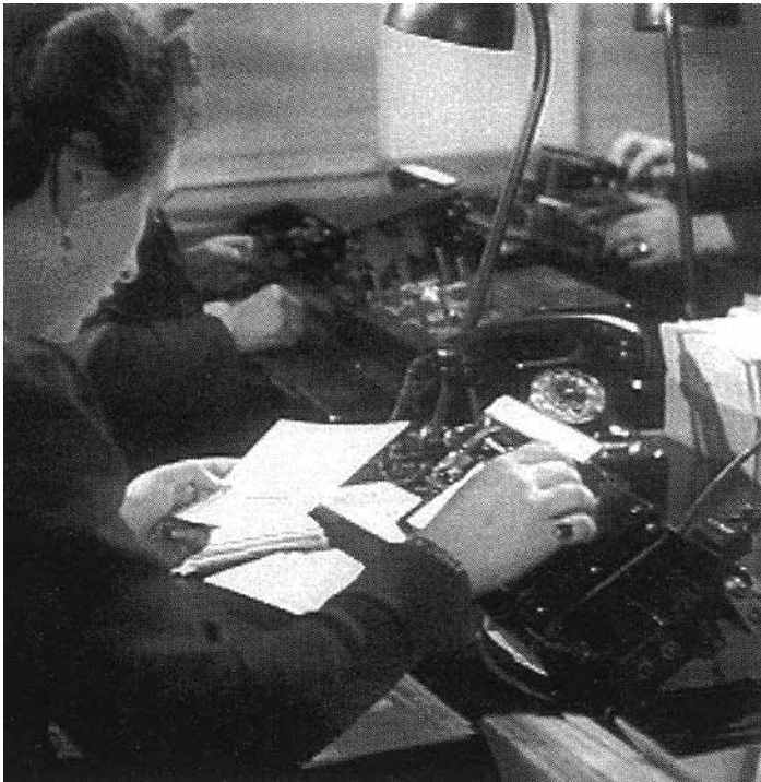
The hand punch card device was used to transfer statistical data to the punch card (film print).
